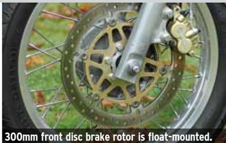
300mm front disc brake rotor is float-mounted.
