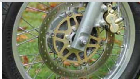
300mm front disc brake rotor is float-mounted.
