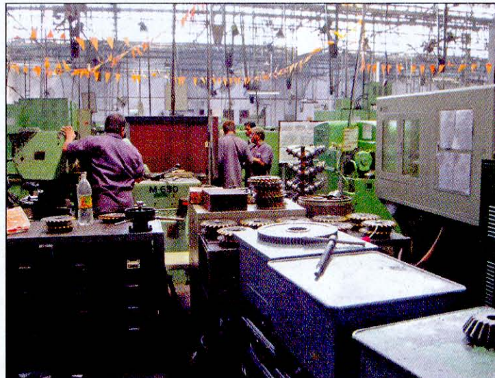
Crown wheels being assembled and inspected at Eicher Engineering's Thane facility
